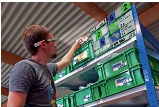
**Fig. 1. Pick by vision picking technology**
