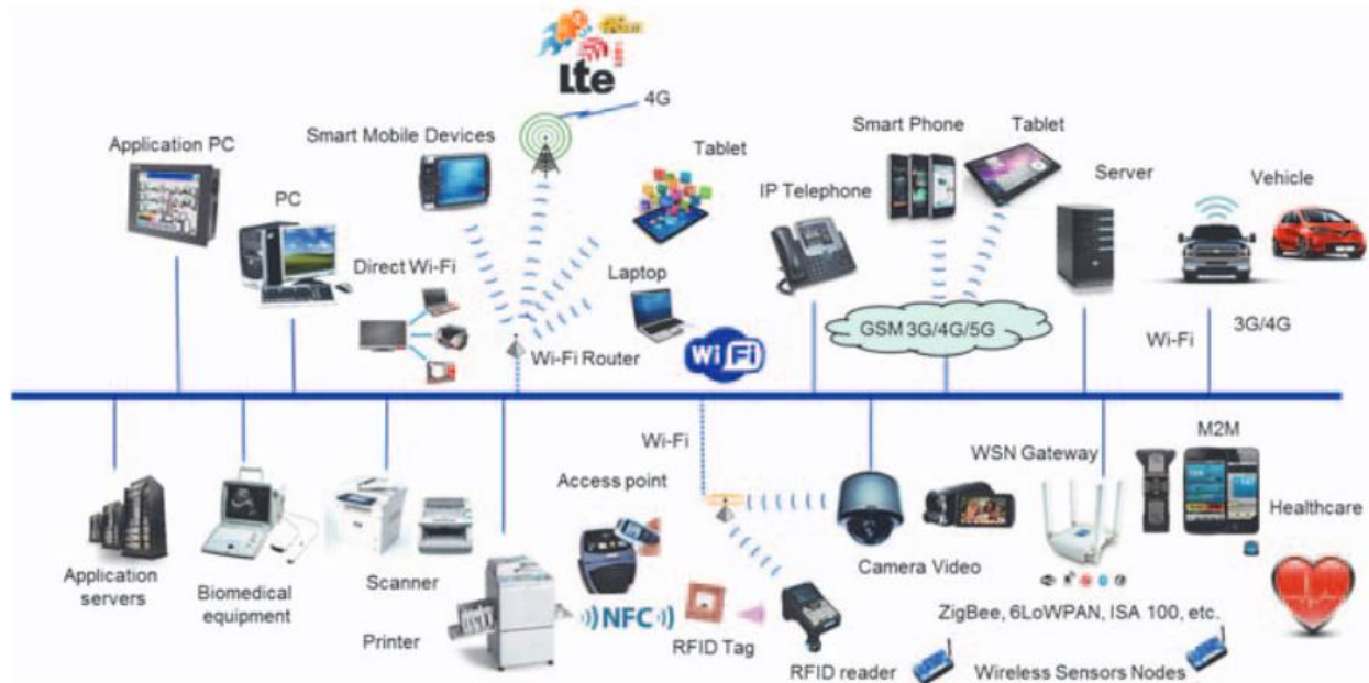
2. ábra: A dolgok internete – IP konvergencia (Forrás: Vermesan O., Friess P. (2013) Internet of Things – Converging Technologies for SMART Environments and Integrated Ecosystems , River Publisher, pp. 13)
