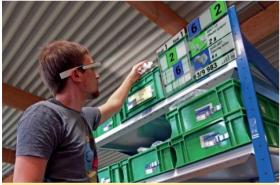
Fig. 1. Pick by vision picking technology
